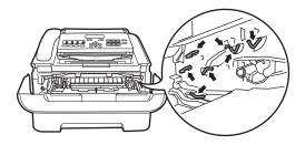
4 Push down the green lock lever and take the toner cartridge out of the drum unit. Clear the jammed paper if there is any inside the drum unit.
