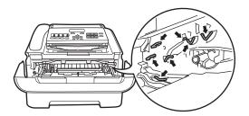
4 Push down the green lock lever and take the toner cartridge out of the drum unit.
