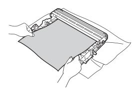
6 Turn the drum unit gear by hand while looking at the surface of the drum roller (1).
