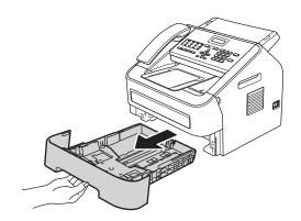
While pressing the green paper-guide release lever, slide the paper guides to fit the paper size you are loading in the tray. Make sure that the guides are firmly in the slots.
