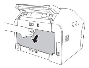
5 Pull down the tabs at the left and right hand sides to open the fuser cover (1).
