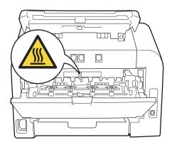
Slowly take out the drum unit and toner cartridge assembly. The jammed paper may be pulled out with the drum unit and toner cartridge assembly, or this may release the paper so you can pull it out from inside of the machine.
