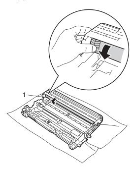
When you have found the mark on the drum that matches the print sample, wipe the surface of the drum roller with a dry cotton swab until the dust or glue on the surface comes off.
