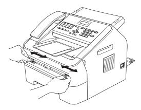
4 Using both hands, put one sheet of paper or one envelope in the manual feed slot until the front edge of the paper or envelope touches the paper feed roller. When you feel the machine pull in the paper, let go.
