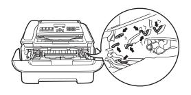
4 Clean the corona wire inside the drum unit by gently sliding the green tab from right to left and left to right several times.
