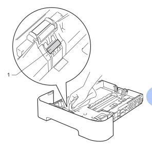
Wipe the two pick-up rollers (1) inside of the machine to remove dust.
