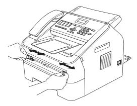
Using both hands, put one piece of A4 or Letter size paper in the manual feed slot until the top edge of the paper touches the paper feed roller. When you feel the machine pull in the paper, let go. The machine will start the Drum Cleaning process.
