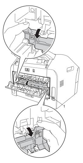
6 Using both hands, gently pull the jammed paper out of the fuser unit.
